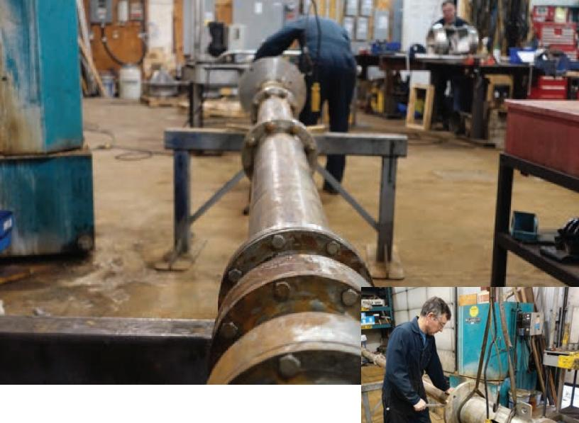
The pump is completely blasted and cleaned to as new condition.
